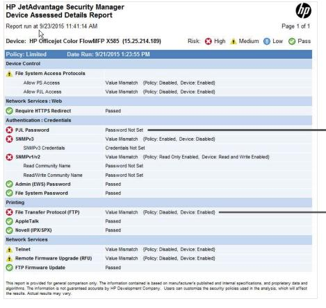
Unconfirmed passwords/ certificates could lead to unauthorized access to the device
